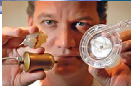
Above: A cutaway view of the VentrAssist LVAD, showing its unique floating impeller, which is the 2.5-inch device's only moving part. Right: The Berlin Heart Pediatric VAD, an external heart device that has been used at Children's Hospital of Pittsburgh of UPMC.
