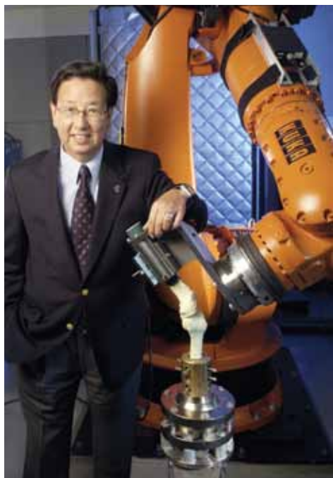
Savio Woo with a robotic/Universal-Force Sensor testing system
