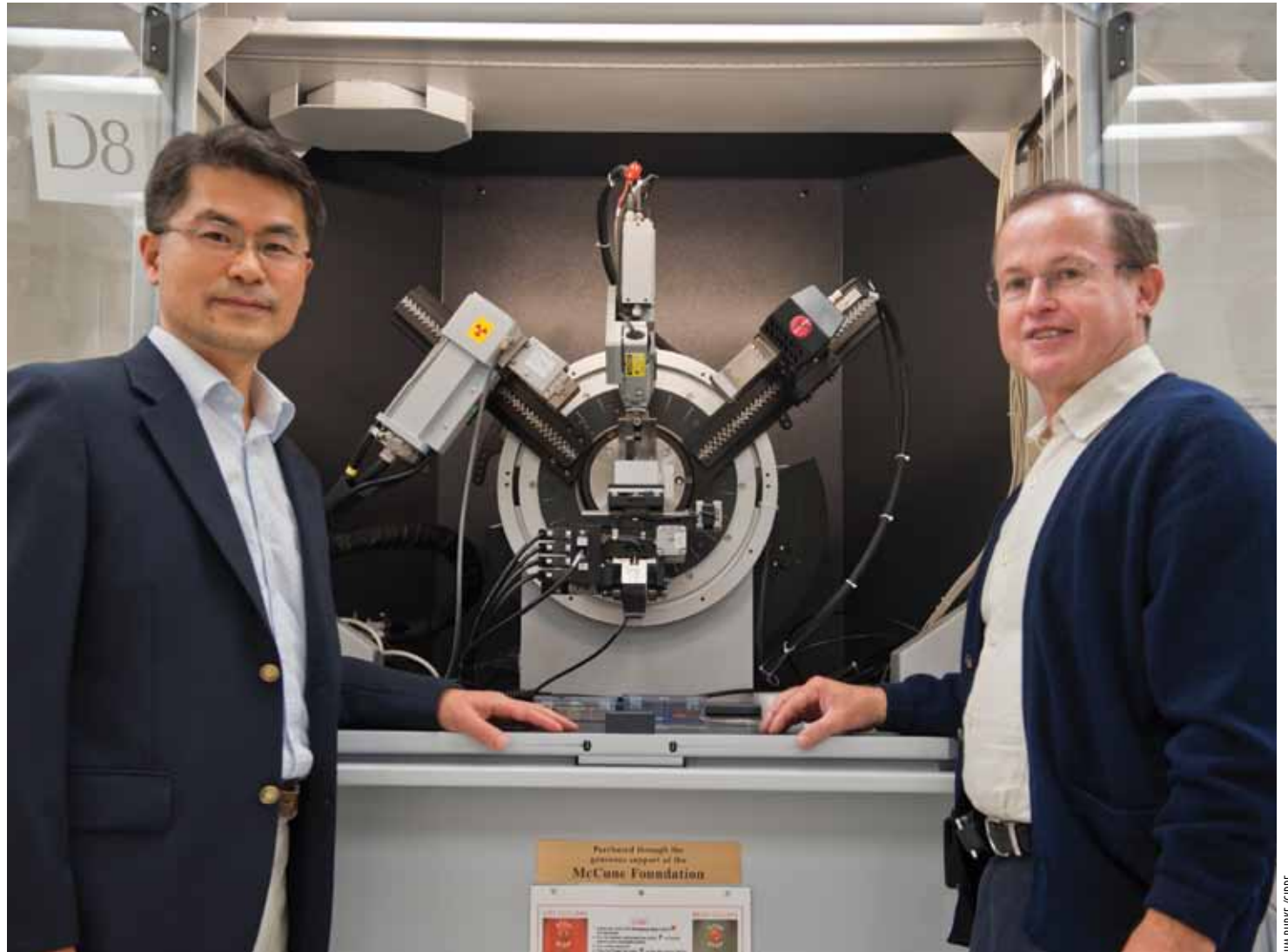
One of the key instruments in Pitt's nano lab is the X-ray diffraction system (above), which analyzes the structural properties of nanomaterials at the atomic or molecular level. The University's Petersen Institute for NanoScience and Engineering (PINSE) has invested almost $12 million to stock its facility with more than two dozen of the most advanced instruments required for high-level nanoscience research. Pictured are Hong Koo Kim (left) and Hrvoje Petek.
