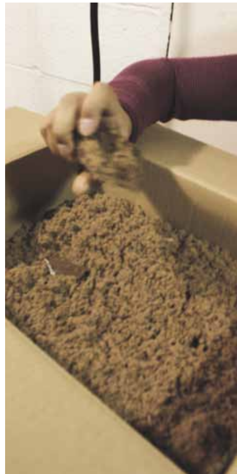
Above: The extractor removes water from the slurry before the food pulp is baked into fertilizer. The water is filtered and then recycled through the pulper. Left: After 18 hours of baking, the food, napkins, chopsticks, and other organic material emerge as nitrogen-rich compost with the feel of sawdust.
