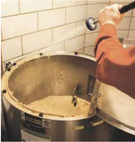
Tod Shoenberger, unit manager for Sodexo, rinses the inside of the pulper, an industrial-sized blender that grinds food and other organic matter into a slurry. In October, Shoenberger used the resulting compost on his home rose garden with excellent results, he said.
