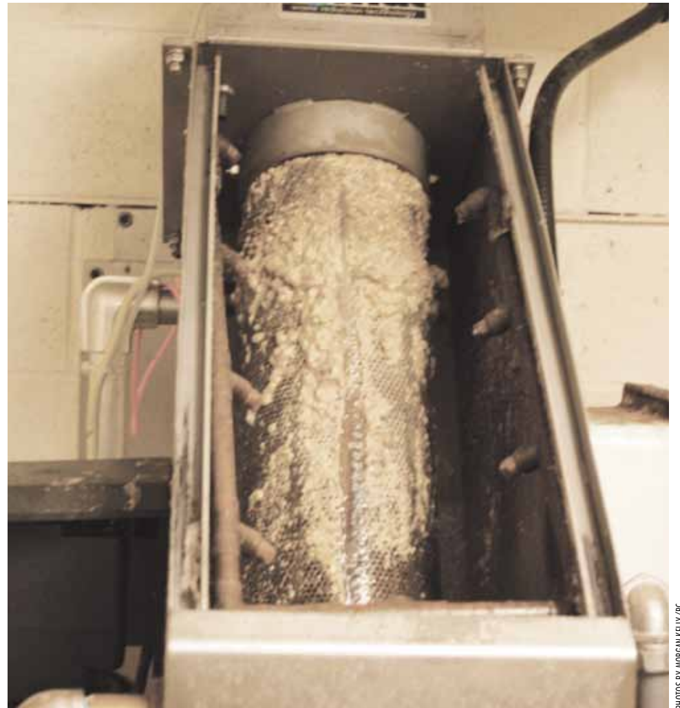
Above: The extractor removes water from the slurry before the food pulp is baked into fertilizer. The water is filtered and then recycled through the pulper. Left: After 18 hours of baking, the food, napkins, chopsticks, and other organic material emerge as nitrogen-rich compost with the feel of sawdust.
